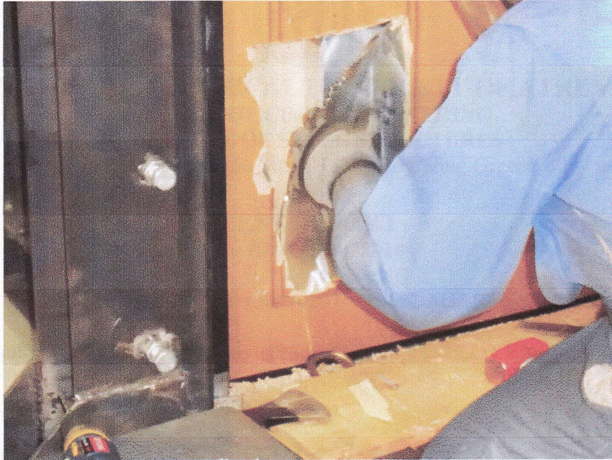
Figure 5 Execution of the main test at following resistance times: a) 4 minutes, b) 10 minutes, c) 12 minutes (continued)
