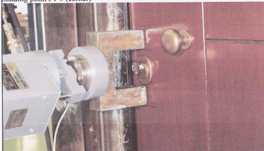
Loading point F3-8 (main lock)
