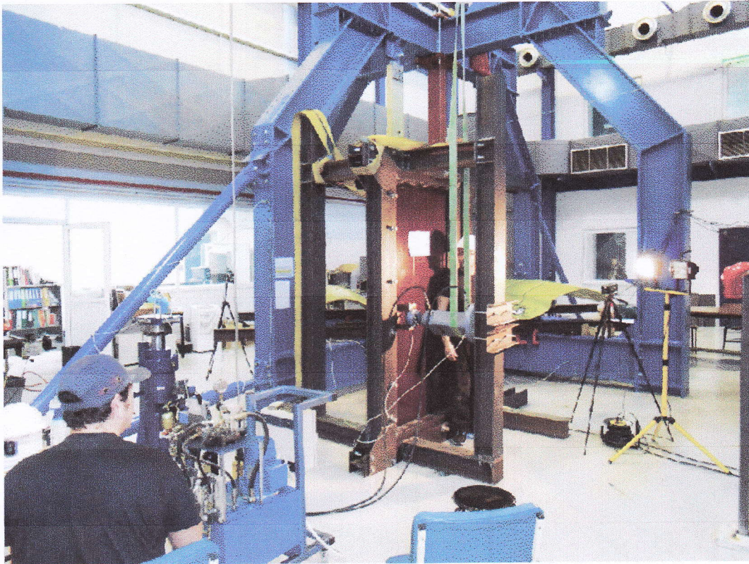
Figure 3 Test rig, hydraulic actuator and loading
